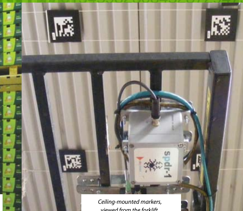
Each pallet movement is tracked through ceiling-mounted markers (dot matrix bar codes) that identify each location in the cool store.
